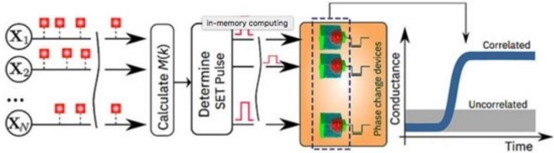
A schematic illustration of the in-memory computing algorithm. Credit: IBM Research
